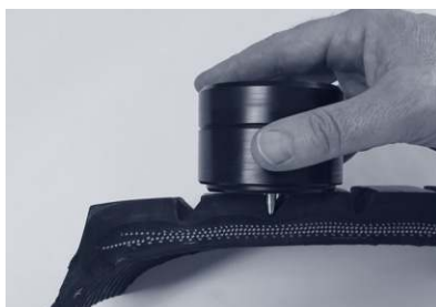
Fig. 4: Measurement of the under-tread thickness in the grooves of the tread up to the steel mesh (max. 10 mm) with probe F 30-T and steel pin.
