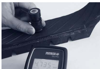
Fig. 6: Measurement of the rubber thickness inside beneath the tread up to the steel mesh (max. 6.5 mm) with probe F10-2.
