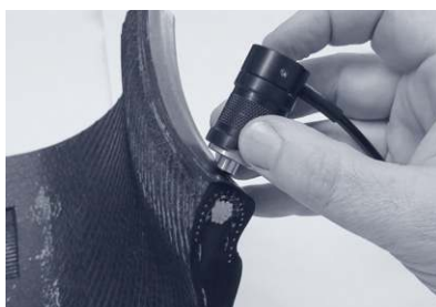
Fig. 7: Measurement of rubber thickness on the bead up to the steel mesh (max. 6.5 mm) with probe F10-3.
