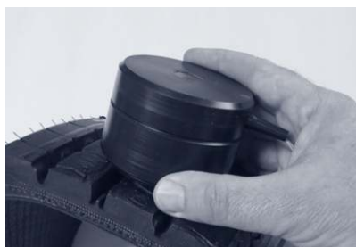
Fig. 3: Measurement of the rubber thickness on the running surface up to the steel mesh (max. 30 mm) with probe F 30-T.
