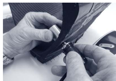
Fig. 8: Measurement of total rubber thickness of the side wall with fabric carcass (max. 10 mm) with probe F10-cp and Fe counter pole.
